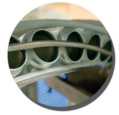
Our Vision Systems inspect the inside can, body, neck and flange areas as well as converted ends for coating voids, wrinkles, creases, puckers, scratches and dents—even mixed labels so rogue cans don't escape your attention. Any differences are flagged, and out-of-spec cans are automatically rejected.
